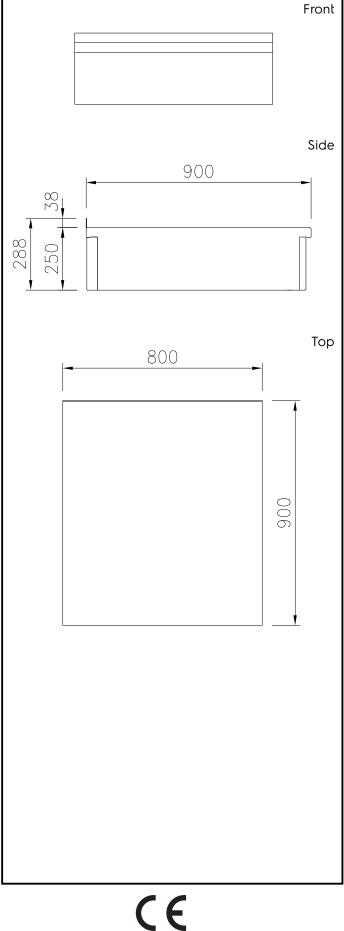
Modular Cooking Range Line thermaline 90 - 800 mm Closed Work top, 1 Side with Backsplash
